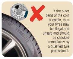
When taking the test, remember to check at least three locations around each tyre. As the test is so guick and easy, stay safe by checking your tyres at least once a month.
